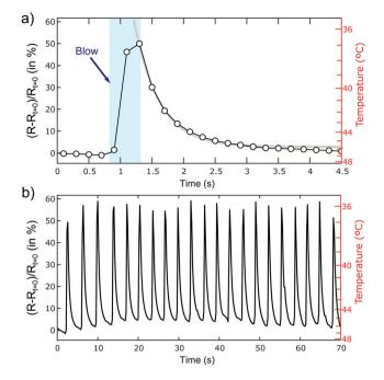
Fig. 5 Response time of WS<sub>2</sub>-on-paper thermoresistive devices upon sudden temperature changes. (a) Resistance change vs. time of a WS<sub>2</sub>-on-paper device subjected to a sudden change in temperature. The device is warmed up to  ${\sim}45~^{\circ}\mathrm{C}$  and at time  $t\sim1$  s a hand pump blows cool air onto the device. (b) 21 blowing cycles to demonstrate the reproducibility of the thermoresistive device.
