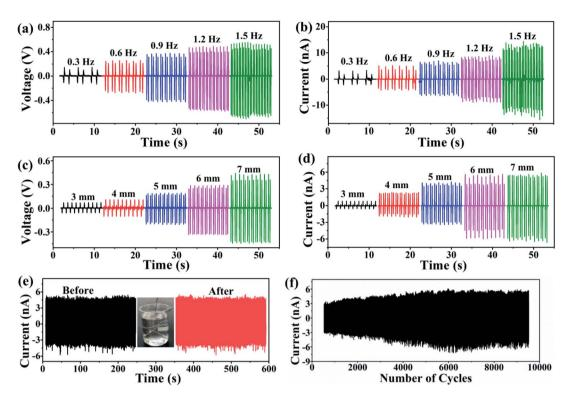
Fig. 3 (a) Output voltage and (b) output current of FTNG under different lateral sliding frequencies. (c) Output voltage and (d) output current of FTNG under different lateral sliding displacements. (e) Output current before and after washing operation. (f) Output current when continually working for 3 hours.
