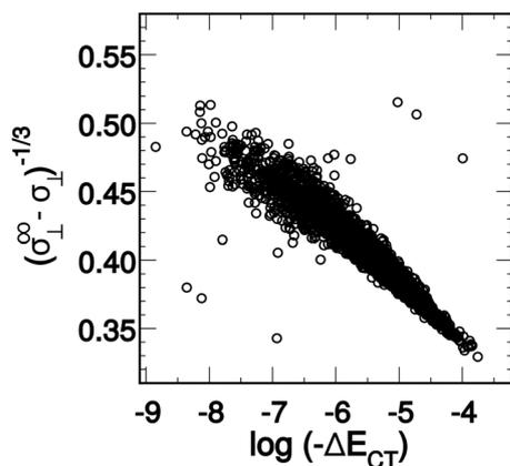
Fig. 1 A derived linear model relating the orthogonal component of the  $^1\text{H}$  shielding tensor in water ( $\sigma_{\perp}$ ) to the stabilization energy due to charge-transfer ( $\Delta E_{\text{CT}}$ ). The shielding tensor component in the limit of a HB-free water molecule is denoted as  $\sigma_{\perp}^{\infty}$ . Reproduced from ref. 17/CC BY.
