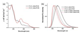
Fig. 1 (a) UV-vis absorption spectra and (b) PL spectra of **tetra-Pt-S** and **tetra-Pt-M** in  $CH_2CI_2$  and PMMA at room temperature.
