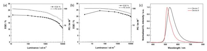
Fig. 3 The EL characteristics of device 7 and device 8; (a) the EQE-PE-luminance characteristics of device 7; (b) the EQE-PE-luminance characteristics of device 8; and (c) the EL spectra of device 8 at a luminance of  $1000 \text{ cd m}^{-2}$ .
