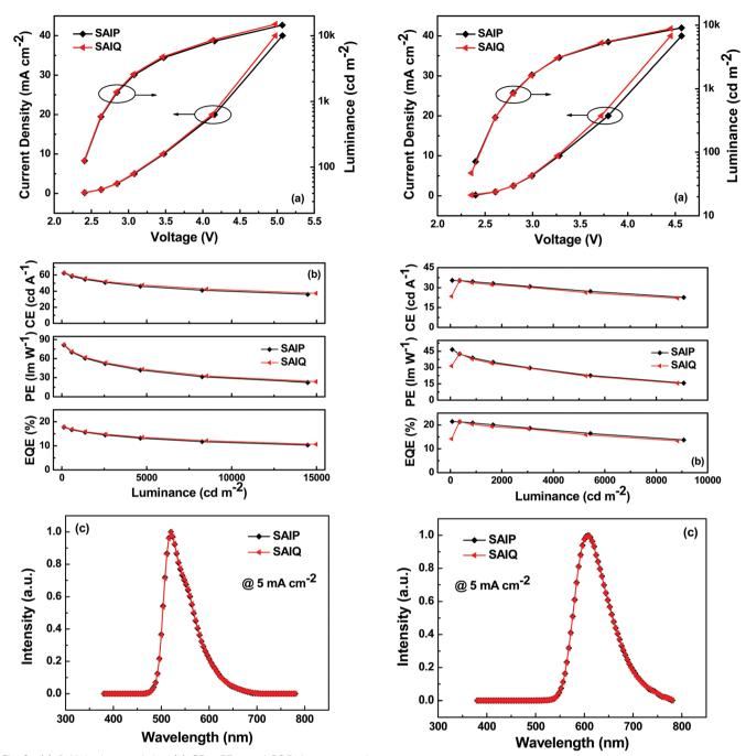
Fig. 8 (a) J-V-L characteristics, (b) CE-, PE-, and EQE-L curves, and (c) EL spectra of the green devices.
