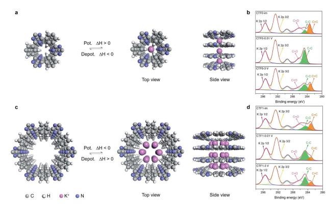
Fig. 4 Simulated  $K^+$  storage mechanisms in CTF-0 (a) and CTF-1 (c) materials.  $\Delta H$  represents the enthalpy change in the corresponding potassiation (Pot.) or depotassiation (Depot.) process. XPS spectra of C 1s of CTF-0 (b) and CTF-1(d), corresponding to the pristine anode after being immersed in electrolyte, in the discharged state of 0.01 V and in the charged state of 3.0 V, respectively.
