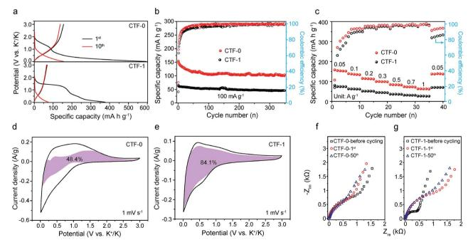
Fig. 3 (a) Discharge/charge curves of the initial and the  $10^{th}$  curves at a current density of 50 mA  $g^{-1}$ ; (b) cycling performance of CTF-0 and CTF-1; and (c) rate capabilities of the CTFs. CV curves and the corresponding pseudocapacitive fractions illustrated by the purple region in (d) CTF-0 and (e) CTF-1. The EIS spectra of (f) CTF-0 and (g) CTF-1 before cycling and at the  $1^{st}$  and  $50^{th}$  cycles.
