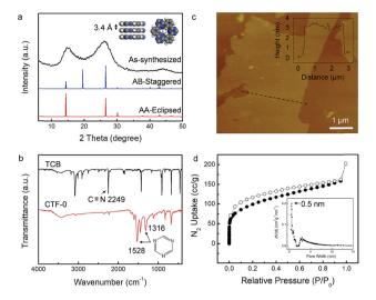
Fig. 2 Structural and morphological characterization of CTF-0. (a) PXRD patterns; (b) FT-IR spectra (TCB stands for the monomer 1,3,5-tricyanobenzene); (c) AFM image and height profile along the black line; and (d)  $\rm N_2$  adsorption isotherms collected at 77 K and (inset) the pore size distribution. The relative pressure ( $P/P_0$ ) range for determination of the CTF-0 BET surface area is from 2.0124  $\times$   $10^{-2}$  to 2.0034  $\times$   $10^{-1}$ .
