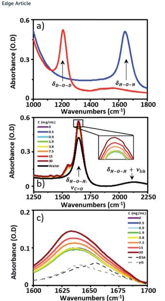
Fig. 1 (a) The IR absorption spectra of  $D_2O$  (red) and  $H_2O$  (blue). (b) IR absorption spectra of serum samples spiked with  $\gamma$ -globulins, pure  $H_2O$  is shown in black. The inset shows an expansion of the tip of the peak due to the H-O-H bending mode of water and the protein amide I band at 1650 cm $^{-1}$ . (c) IR absorption spectra of serum spiked with  $\gamma$ -globulins from (b) following subtraction of the  $H_2O$  spectrum.
