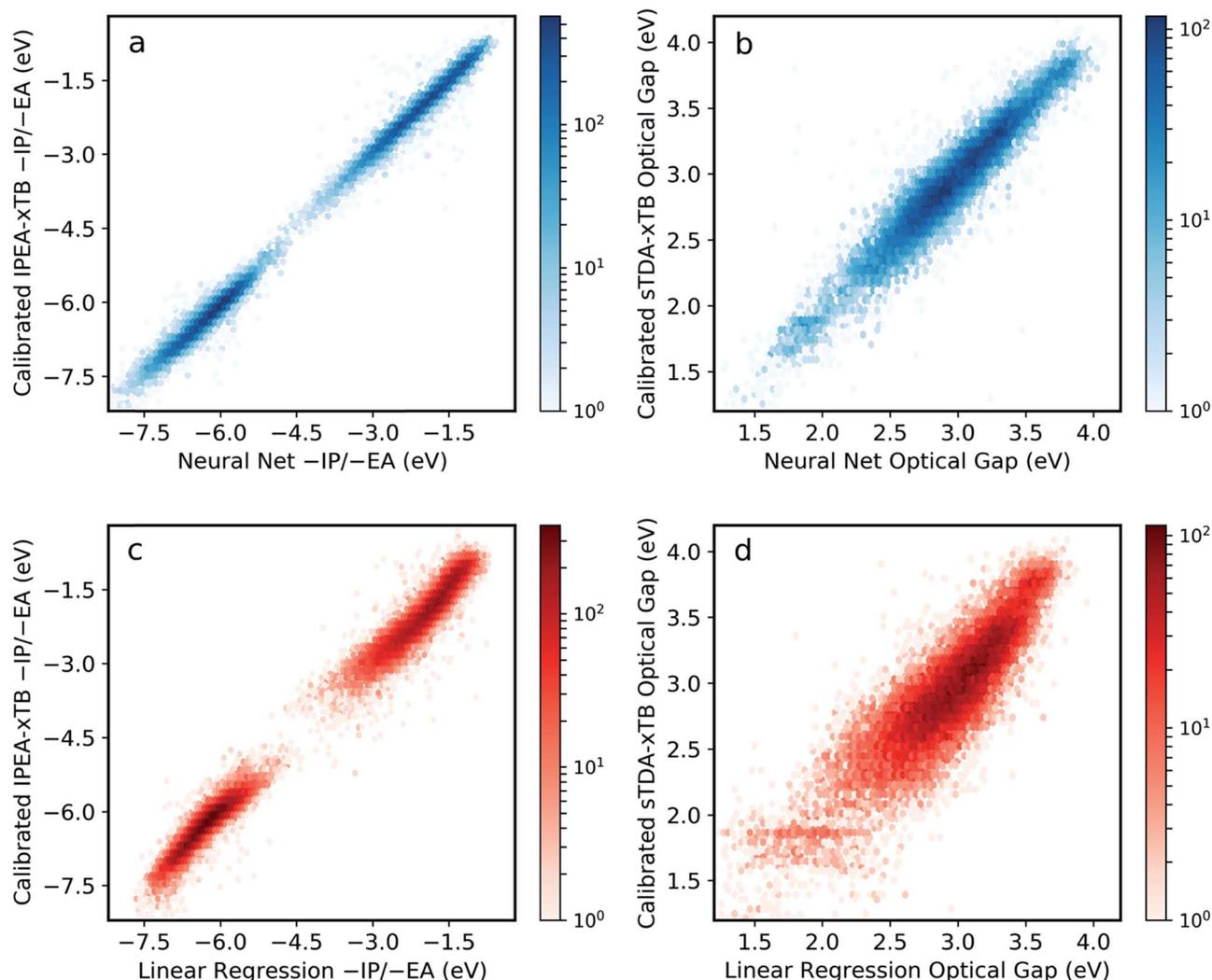
Fig. 2 Performance of neural network model when predicting (a)  $-IP$  and  $-EA$ , (b) optical gap ( $S_0 \rightarrow S_1$  excitation energy) values derived from calibrated IPEA-xTB and sTDA-xTB, respectively shown as 2D histograms (dark red (high) – light red (low) density). For comparison, the performance of a linear regression model is also given (c and d). All properties correspond to copolymer compositions not used during the training phase.
