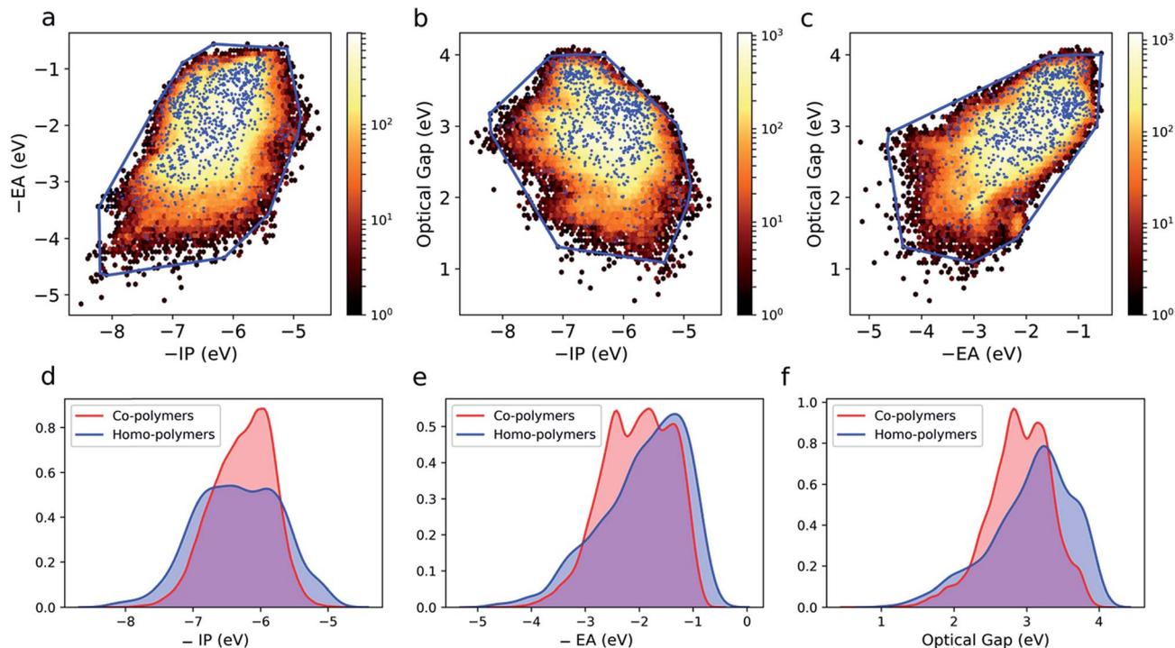
Fig. 3 2D histograms of copolymer property spaces spanned by (a)  $-IP$  and  $-EA$ , (b)  $-IP$  and optical gap, (c)  $-EA$  and optical gap. In each case, the property space spanned by copolymers (dark red (low) – yellow (high) density) and homopolymers (blue dots) is shown. The property space enclosed by the homopolymers is also shown as a convex hull (blue line). Kernel density estimates (KDE) of (d)  $-IP$ , (e)  $-EA$  and (f) optical gap for both homo- and copolymers.
