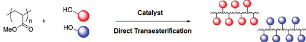
Fig. 14 Transesterification-based synthetic strategy to functional polyacrylates. Reproduced from ref. 136 with permission from WILEY-VCH Verlag GmbH & Co., copyright [2017].
