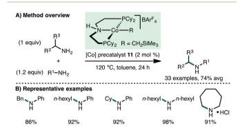
Scheme 15 Co-Catalysed cross coupling of 1° and 2° amines (Zheng,
