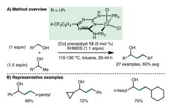
Scheme 21 Co-Catalysed cross coupling of 2° and 1° alcohols (Kempe).
