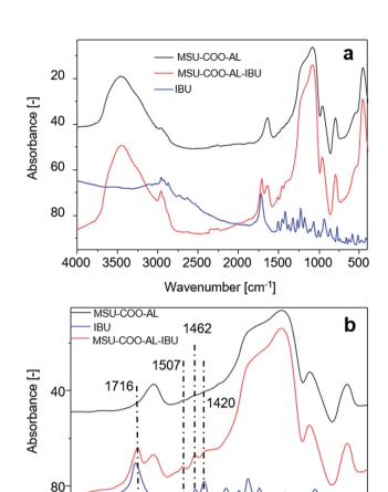
Fig. 6 (a) FT-IR spectra of samples MSN-COO-Al, MSN-COO-Al-IBU and ibuprofen (IBU); (b) magnification of (a) in the range between 2000 and 750  $\rm cm^{-1}$ .
