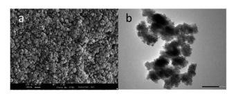
Fig. 2 (a) Electron scanning microscopy (SEM) image of the MSN sample and (b) TEM micrograph of the same sample.
