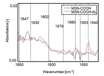
Fig. 4 FT-IR spectra of MSN-COOH and MSN-COOH-AL functionalized silica before and after the AL loading step in the range of  $1650-1450~{\rm cm}^{-1}$ .
