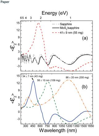
Fig. 2 (a) SE measurement of the sample with Ga NPs of 41 nm radius and reference samples of sapphire and the as-grown MoS<sub>2</sub>/sapphire. (b) SE measurements of different Ga NPs/MoS<sub>2</sub> samples where the LSPR shift with the NP radius can be observed.
