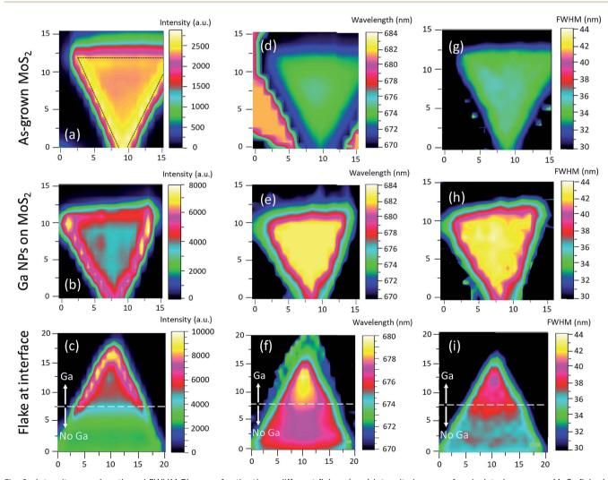
Fig. 6 Intensity, wavelength and FWHM PL maps for the three different flakes. (a-c) Intensity images of an isolated as-grown MoS<sub>2</sub> flake (a), a totally covered  $MoS_2$  flake with Ga NPs (b), and a half covered with Ga NPs (c). (d-f) Images corresponding to the wavelength peak center for the same flakes shown in (a-c). (q-i) Images corresponding to the FWHM of the PL peak of the same flakes shown in (a-c). Axes indicate the horizontal and the vertical distance in um.
