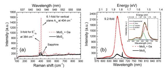
Fig. 3 (a) Raman and (b) PL spectra of a MoS<sub>2</sub> sample with and without Ga NPs in order to observe the plasmonic enhancement in both cases (excitation at 532 nm). The PL spectra of the pristine MoS<sub>2</sub> sample is analyzed in the inset of (b) via fitting with a trion and two excitons.
