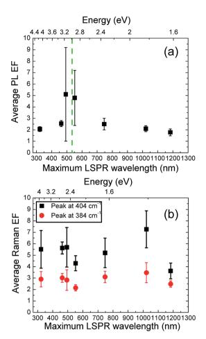
Fig. 4 (a) Average PL peak intensity EF of monolayer MoS<sub>2</sub> as a function of the LSPR position of Ga NPs. The green line represents the laser wavelength, 532 nm. (b) Average Raman EF of monolayer MoS<sub>2</sub> peaks at 384 and 404  $cm^{-1}$  as a function of the LSPR position of Ga NPs. Error bars indicate the standard deviation.
