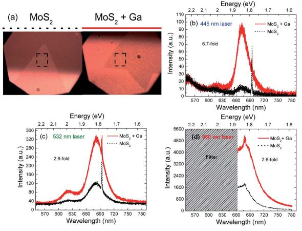
Fig. 7 (a) Microscope images of the  $MoS_2$  flake without (left) and with Ga NPs (right). Frames indicate the measurement point. PL spectra of monolayer  $MoS_2$  with and without Ga NPs for the same flake with laser wavelengths of 445 nm (b), 532 nm (c) and 660 nm (d). The EF and peak wavelength are also indicated for each case. The maximum LSPR wavelength of the deposited Ga NPs is 463 nm.
