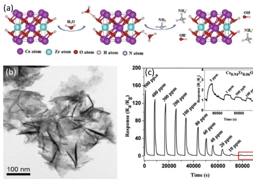
Fig. 18 (a) Schematic diagrams of the NH<sub>3</sub> reaction mechanism on the surface of Ce<sub>0.94</sub>Zr<sub>0.06</sub>O<sub>2</sub> nano-sheets; (b) TEM image of porous Ce<sub>0.94</sub>Zr<sub>0.06</sub>O<sub>2</sub> nano-sheets; (c) response/recovery curves of the porous Ce<sub>0.94</sub>Zr<sub>0.06</sub>O<sub>2</sub> nanosheet based sensor to NH<sub>3</sub>.<sup>127</sup> Copyright 2018, Elsevier.
