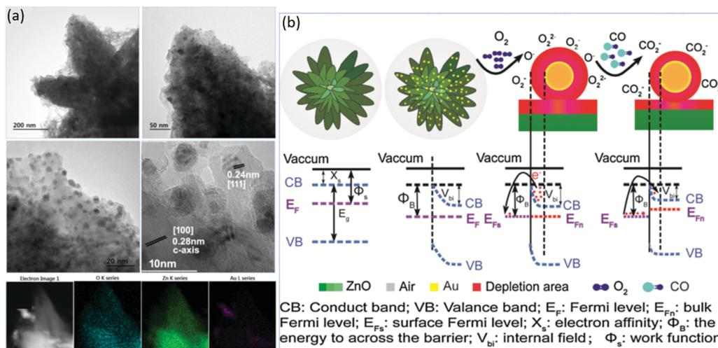
Fig. 14 (a) TEM images and element mapping of Au/ZnO nanostars; (b) energy band diagrams of ZnO and Au/ZnO nanostars before and after CO exposure.<sup>113</sup> Copyright 2017, Elsevier.
