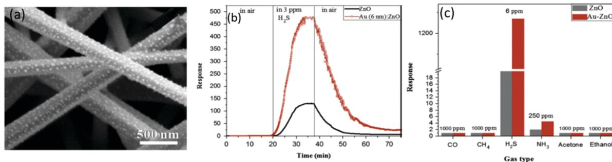
Fig. 16 (a) SEM image of Au/ZnO nanorods; (b) response/recovery curves of the Au/ZnO nanorod-based sensor and pristine ZnO nanorod-based sensor to 3 ppm H<sub>2</sub>S at room temperature; (c) responses of the Au/ZnO nanorod-based sensor and pure ZnO nanorod-based sensor to different gases.<sup>257</sup> Copyright 2015, Elsevier.
