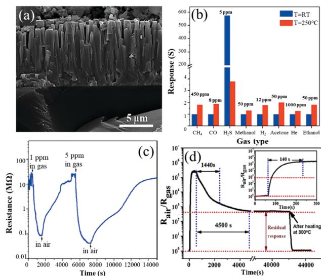
Fig. 4 (a) Cross-section SEM image of vertically aligned  $\text{ZnO}$  rods; (b) selectivity of the sensor at 25 °C and 250 °C; (c) response/recovery curves to 1 and 5 ppm  $\text{H}_2\text{S}$  at room temperature.<sup>71</sup> Copyright 2015, Elsevier. (d) The response/recovery curve at 50 ppm  $\text{H}_2\text{S}$  gas at room temperature.<sup>101</sup> Copyright 2017, Elsevier.
