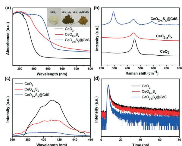
Fig. 4 (a) UV-visible diffuse reflectance absorption spectra, (b) Raman spectra, (c) photoluminescence spectra, and (d) TRPL spectra of the  $\text{CeO}_2$ ,  $\text{CeO}_{2-x}\text{S}_x$  and  $\text{CeO}_{2-x}\text{S}_x@\text{CdS}$  samples.
