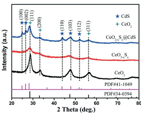
Fig. 1 XRD patterns of the  $\text{CeO}_2$ ,  $\text{CeO}_{2-x}\text{S}_x$  and  $\text{CeO}_{2-x}\text{S}_x@\text{CdS}$  samples.
