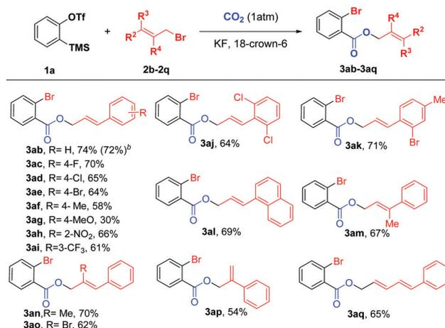
Scheme 3 <sup>a</sup>Reaction conditions: **1a** (0.24 mmol), **2** (0.2 mmol),  $\text{CO}_2$  (1 atm), KF (2.4 equiv.), 18-crown-6 (2.4 equiv.),  $\text{CF}_3\text{-Ph}$  (1 mL),  $-10$  to  $10$  °C for 12 h. <sup>b</sup>Reaction conditions: **1a** (1.2 mmol), **2** (1 mmol),  $\text{CO}_2$  (balloon), KF (2.4 equiv.), 18-crown-6 (2.4 equiv.),  $\text{CF}_3\text{-Ph}$  (5 mL),  $-10$  to  $10$  °C for 12 h.
