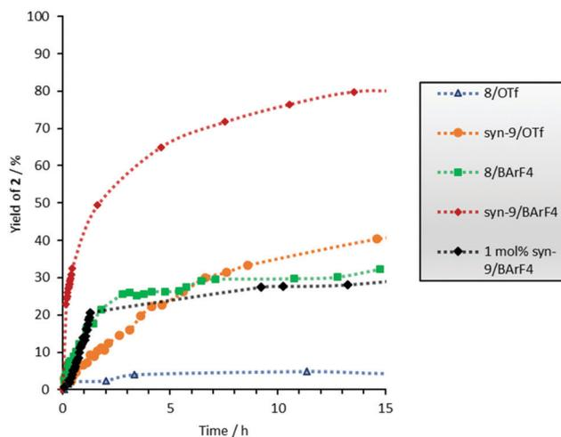
Fig. 4 <sup>1</sup>H-NMR yield vs. time profile for the formation of cyclopentenone **2**. The error is approximately 5%. *c*<sub>0</sub>(**1**) = 15.4 mM.
