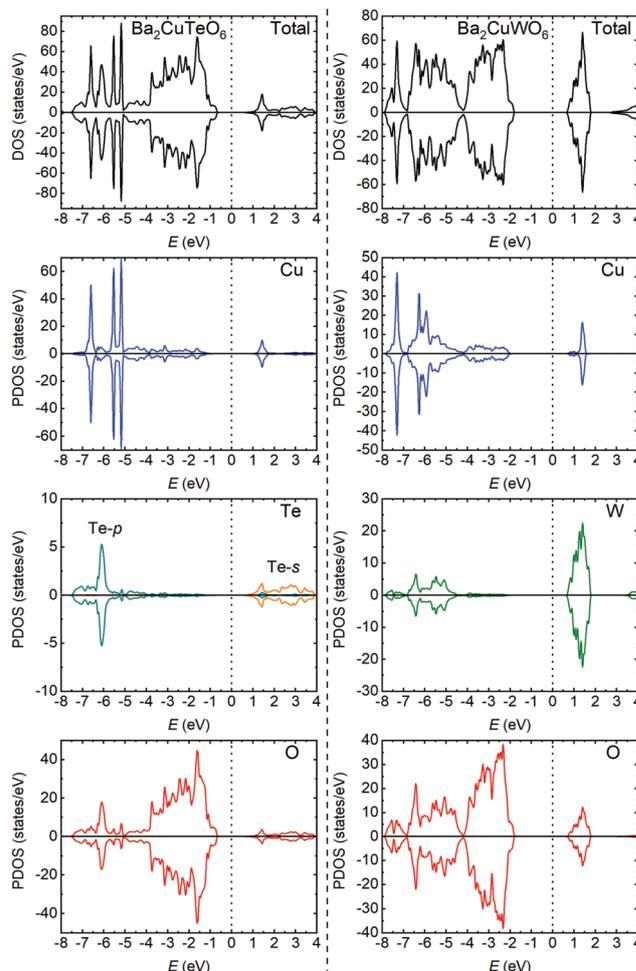
**Fig. 2** Total and partial density of states plots for  $\text{Ba}_2\text{CuTeO}_6$  (left) and  $\text{Ba}_2\text{CuWO}_6$  (right). Both compounds are antiferromagnetic insulators. The moderate Te 5p/5s–O 2p hybridisation and stronger W 5d–O 2p hybridisation are seen in the Te/W and O PDOS plots.
