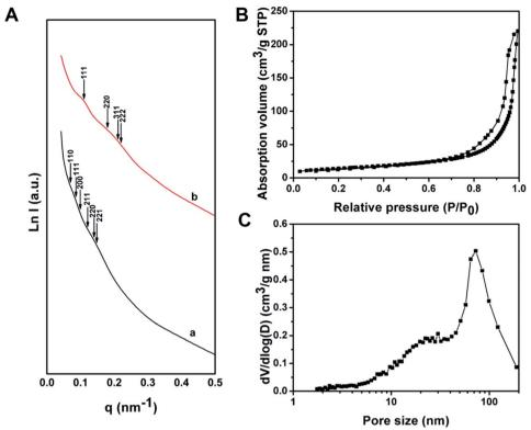
Fig. 3 (A) SAXS patterns of (a) as-made  $Al^{3+}$ -based gel/PEO-b-PMMA composites prepared by the vesicle-aggregation-assembly approach and (b) ordered mesoporous alumina obtained after calcination at 900 °C in air. (B) Nitrogen sorption isotherms and (C) pore size distribution of the ordered mesoporous alumina prepared by the vesicle-aggregation-assembly approach after calcination at 900 °C in air.
