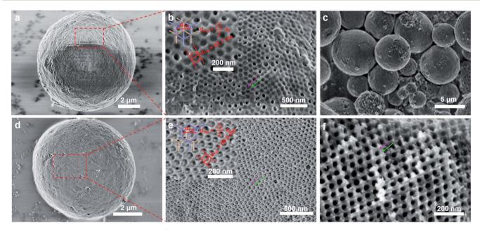
Fig. 1 FESEM images of (a, b) the as-made  $Al^{3+}$ -based gel/PEO-b-PMMA composite microsphere prepared by the vesicle-aggregation-assembly approach, (c-e) ordered mesoporous alumina microspheres and (f) its fragment obtained after calcination at 900 °C in air. The insets in (b) and (e) show enlarged SEM images and corresponding theoretical stick models, respectively.
