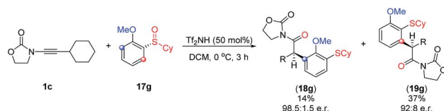
Scheme 5 Asymmetric rearrangement with chiral enantiopure sulfoxides.
