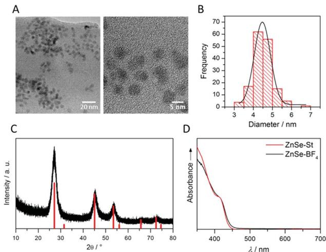
Fig. 2 Characterisation of ligand-free ZnSe QDs (ZnSe-BF<sub>4</sub>): (A) transmission electron micrographs with (B) corresponding particle size distribution. (C) Powder X-ray diffractogram overlaid with cubic zinc blende ZnSe reference (PDF 01-071-5978); (D) UV-vis spectrum compared to ZnSe-St.
