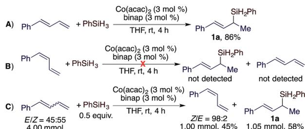
Scheme 4 Hydrosilylation of an *E/Z*-mixture of dienes using Co(acac)<sub>2</sub>/binap.
