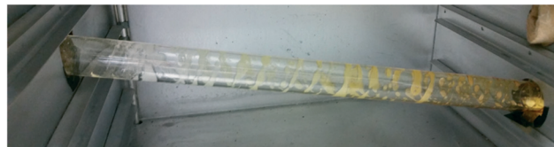
Fig. 6 The helix effect seen as the reaction is occurring on the inner surface of the work-tube. The colour change from colourless to yellow can be seen as the reaction occurs. The opacity of the solution appears to change; this is due to the formation of gas bubbles which are escaping.
