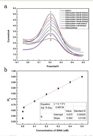
Fig. 6 (a) Differential pulse voltammograms plots of  $0.2 \text{ M} \text{ K}_3 [\text{Fe}(\text{CN})_6]$  at pDNA (500 nM) immobilized GQDs modified GCE in 1.0 M KCl and that after hybridization with different concentrations of HBV-DNA (tDNA). (b) The plot of the peak current against the concentration of HBV-DNA.
