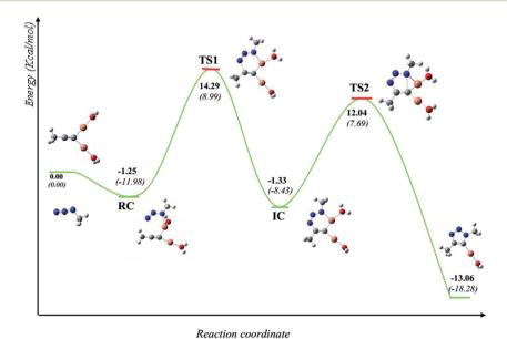
Fig. 6 Schematic representation (energy (kcal mol<sup>-1</sup>) vs. reaction coordinate) of the reaction of copper(i)-catalyzed 32CA between methyl azide and propyne (bold numbers for gas phase and numbers between brackets for water as reaction medium).
