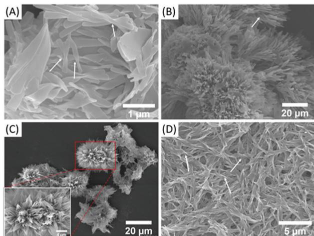
Fig. 3 SEM images of **trans-C<sub>5</sub>-Chol** in (A) DMF, (B) acetone, (C) EA and (D) DCM/EA (1/2, v/v); inset: partial enlarged view.
