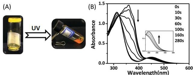
Fig. 5 (A) Photos showing gel-sol transition of *trans*-C<sub>5</sub>-Chol in DMF ( $c = 62$  mM) after 15 min of UV irradiation ( $90$  mW  $\text{cm}^{-2}$ ,  $365$  nm). (B) UV-Vis spectra of *trans*-C<sub>5</sub>-Chol in DMF solution ( $c = 0.1$  mM) with different UV irradiation time ( $0.25$  mW  $\text{cm}^{-2}$ ,  $365$  nm).
