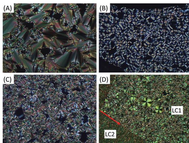
Fig. 2 Textures of *trans*-C<sub>n</sub>-Chol observed by POM upon cooling from isotropic phase. (A) *trans*-C<sub>0</sub>-Chol at 25 °C; (B) *trans*-C<sub>1</sub>-Chol at 25 °C; (C) *trans*-C<sub>3</sub>-Chol at 25 °C; (D) *trans*-C<sub>5</sub>-Chol at 145 °C (the second phase LC2 started to grow from the left side). These typical fan-shaped textures indicate SmA phase. In (D) LC1 is SmA, while LC2 is a crystalline phase (see text).
