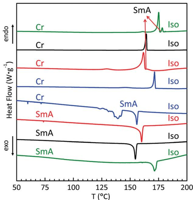
Fig. 1 DSC thermograms of *trans*-C<sub>0</sub>-Chol (green lines), *trans*-C<sub>1</sub>-Chol (black lines), *trans*-C<sub>3</sub>-Chol (red lines) and *trans*-C<sub>5</sub>-Chol (blue lines) upon the first heating (4 upper curves) and first cooling (4 lower curves) cycle at a rate of 2 °C min<sup>-1</sup>. Samples are solids obtained by recrystallization after synthesis.
