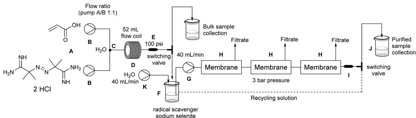
**Fig. 8** a) System for the synthesis and purification of poly(acrylic acid); A: Reagent feed lines, B: Piston pumps, C: Mixer, D: Reactor, E: Backpressure regulator, F: Sample collection, G: Peristaltic pump to feed membranes, H: Ultrafiltration membranes, I: Pressure regulator, J: Filtrate of purification, K: HPLC pump used to maintain the sample volume.
