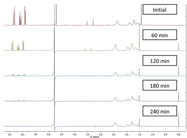
**Fig. 1** <sup>1</sup>H NMR batch dialysis results shown for individual samples at different time intervals.
