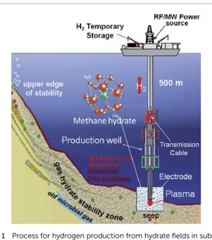
Fig. 1 Process for hydrogen production from hydrate fields in subsea sites using the plasma from the in-liquid method. Reproduced from Rahim and coworkers.<sup>2</sup> Copyright 2015 by Elsevier.
