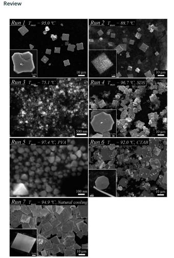
Fig. 12 SEM images of single crystals of a tin oxide SnO plate synthesized by in-liquid plasma under different reaction temperatures, dispersant and cooling conditions. Reproduced from Saito *et al.*<sup>94</sup> Copyright 2012 by the American Chemical Society.
