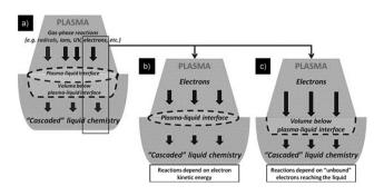
Fig. 4 Schematic diagram of three different types of plasma in-liquid conditions (PiLC): (a) gas-phase species and plasma-radiation-induced liquid reactions at the plasma-liquid interface; (b and c) electrons from the plasma can initiate non-equilibrium reactions in the liquid phase where both electron energy distribution (b) and electron density play an important and distinct role (c). Reproduced from Mariotti et al. 19 Copyright 2012 by WILEY-VCH.
