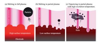
Fig. 13 Images of (a) a wide-area plasma; (b) a partial plasma; and (c) the volatilization of a metal electrode by partial plasma under high temperature conditions. Reproduced from Saito *et al.*<sup>99</sup> Copyright 2014 by the American Institute of Physics.
