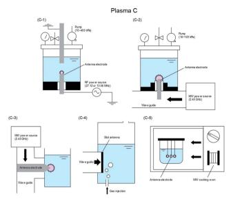
Fig. 8 Typical electrode configuration for Plasma C: (C-1) RF applied in-liquid plasma system under vacuum condition; 129-140 (C-2) MW applied in-liquid plasma system under vacuum condition;134,141-149 (C-3) MW-induced in-liquid plasma system under atmosphere condition;150,151 (C-4) slot-excited MW discharge in-liquid plasma system under atmosphere condition;152 and (C-5) in-liquid plasma generation system with a MW oven. 153,154 Modified with permission from ref. 23. Copyright 2015 by Hindawi.
