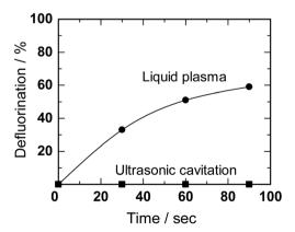
**Fig. 20** Defluorination yields (%) from the degradation of aqueous PFOA solutions (0.01 mM) by ultrasonic cavitation alone and by the microwave discharge in-liquid plasma method under simultaneous ultrasonic cavitation (MW power, 220 W; power for cavitation, 90 W). Reproduced from Horikoshi *et al.* <sup>156</sup> Copyright 2017 by Elsevier.
