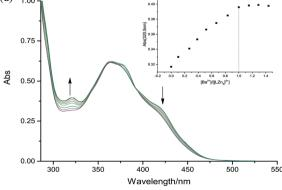
Fig. 2 (a) UV-vis spectrum of the free ligand in  $CHCl_3/CH_3OH$ ; (b) the changes in the Zn(II)-L complex upon addition of  $Ca(OAc)_2 \cdot H_2O$ ; (c) the changes in the Zn(II)-L complex upon addition of Sr(OAc)<sub>2</sub>·H<sub>2</sub>O; (d) the changes in the Zn(II)-L complex upon addition of Ba(OAc)<sub>2</sub>.
