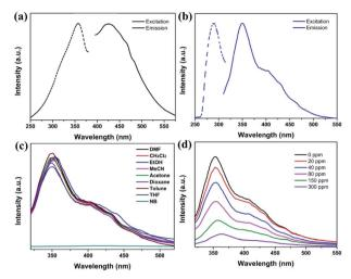
Fig. 2 Excitation (dot lines) and emission (solid lines) spectra of the free  $\rm H_3TATMA$  ligand (a) and 1 dispersed in DMF (b). (c) Luminescent intensity of 1 crystal powder after immersing in DMF with 600 ppm of different analytes for about 2 minutes at room temperature upon excitation at 292 nm. (d) The emission spectra of 1 titrated with NB in DMF for about 2 minutes. 4.0 mg of 1 crystal powder was dispersed in 3.0 mL DMF.
