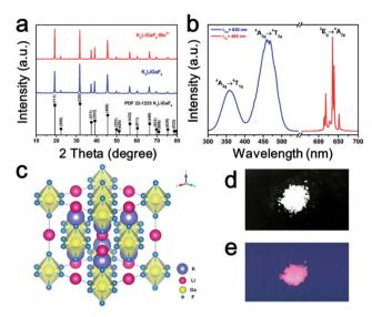
Fig. 1 (a) XRD patterns of  $K_2LiGaF_6$  and  $K_2LiGaF_6$ :Mn<sup>4+</sup>, (b) PLE and PL spectra of  $K_2LiGaF_6$ :Mn<sup>4+</sup>, (c) structure diagram, (d) phosphor under natural light and (e) phosphor under UV-light.
