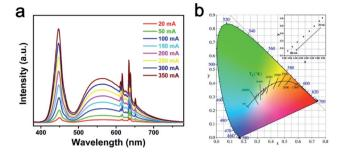
Fig. 5 (a) Electroluminescence spectra and (b) CIE chromaticity diagram of fabricated white LED under various drive currents.
