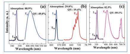
Fig. 7 The excitation lines and emission spectra of the as-prepared samples (a) CAZO:0.5%  $\mathrm{Bi}^{3+}$ , (b) CAZO:0.5%  $\mathrm{Mn}^{4+}$ , and (c) CAZO:1%  $\mathrm{Bi}^{3+}$ ,0.5%  $\mathrm{Mn}^{4+}$  for measurement of the quantum yield using an integrating sphere.
