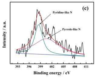
Fig. 2  $\,$  XPS survey of MWCNTs-NS (a) and high resolution XPS of S $_{\rm 2p}$  (b) and N $_{\rm 1s}$  (c).
