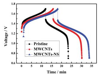
Fig. 6 The 10<sup>th</sup> charge-discharge curves of the cell using the MWCNTs samples as a catalyst in the positive side at a current density of 50 mA cm
