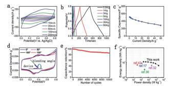
Fig. 5 (a) CV and (b) GCD curves of the symmetric SC in 1.0 M  $H_2SO_4$ electrolyte in a two-electrode system. (c) Specific capacitances at various current densities. (d) CV curves of the GP@cc-based flexible SC at different bending angles. (e) Cycling behavior of the SC device at a current density of 5 A  $g^{-1}$ . (f) Ragone plot of the SC device.
