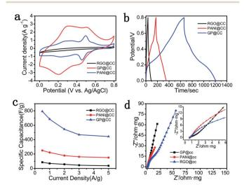
Fig. 3 Electrochemical characterization of rGO@cc, PANI@cc and GP@cc electrodes in a  $1 \text{ M H}_2\text{SO}_4$  electrolyte, three-electrode system. (a) CV curves at a scan rate of 5 mV s<sup>-1</sup>. (b) Galvanostatic charge/discharge curves at a current density of  $1 \text{ A g}^{-1}$ . (c) Specific capacitances *versus* current densities. (d) Nyquist plots with inset showing close-up views of the high-frequency regime.
