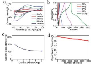
Fig. 4 Electrochemical performance of the GPacc composite. (a) CV curves at different scan rates in a potential range from 0 to 0.8 V and (b) Galvanostatic charge/discharge curves of the GP@cc composite at various current densities in 1 M H<sub>2</sub>SO<sub>4</sub> aqueous solution in a threeelectrode system; (c) specific capacitance at different current densities; (d) capacitance retention over 10 000 cycles at 5 A g<sup>-1</sup>
