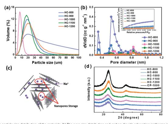
Fig. 4 (a) The particle size distribution of the materials. (b) The pore size distribution and carbon dioxide adsorption isotherms in the inset. (c) Schematic representation of Na ion storage mechanisms in hard carbon (d) XRD patterns of different hard carbon samples.
