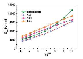
Fig. 7 The relationship between  $Z_{\rm re}$  and  $\omega^{-1/2}$  at low frequencies of HC-1000 electrode.
