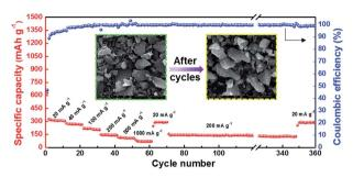
**Fig. 8** Discharge capacities of HC-1000 at different current densities of 20, 40, 100, 200, 500 and 1000 mA  $g^{-1}$ , respectively. A long-term cycling performance is recorded from the 70<sup>th</sup> to the 350<sup>th</sup> cycles at 200 mA  $g^{-1}$  and SEM images of the HC-1000 electrodes before and after 360 cycles.
