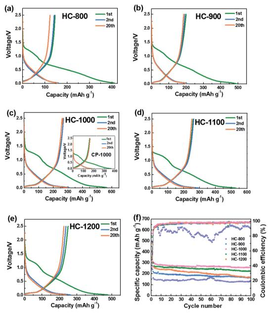
Fig. 5 Discharge-charge profiles of hard carbons at 20 mA  $g^{-1}$  (a) HC-800 (b) HC-900 (c) HC-1000 and CP-1000 (d) HC-1100, and (e) HC-1200, (f) cycling performance of HC electrodes tested at 20 mA  $g^{-1}$ , the voltage range is between 0.01 and 2.5 V.
