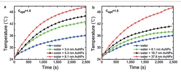
Fig. 9 The temperature changes with time for Au NPs fluids from G1 (a) and G2 (b) under 1.5 kW  ${
