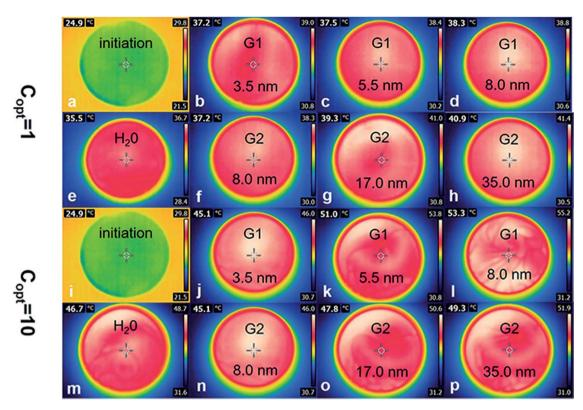
Fig. 7 The temperature of pure water and Au NPs nanofluids with different diameters before and after  $\sim$  2000 s solar illumination under 1 kW m<sup>-2</sup> (a)–(h) and 10 kW m<sup>-2</sup> solar illumination (i)–(p), respectively.
