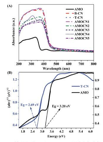
Fig. 4 (A) UV-Vis diffuse reflectance spectra of AMO, B-CN, T-CN, and Ag<sub>2</sub>MoO<sub>4</sub>/g-C<sub>3</sub>N<sub>4</sub> heterojunctions (AMOCN1, AMOCN2, AMOCN3, AMOCN4, and AMOCN5); (B) a plot of  $(\alpha h \nu)^{1/2}$  versus the bandgap (eV) for T-CN and AMO.
