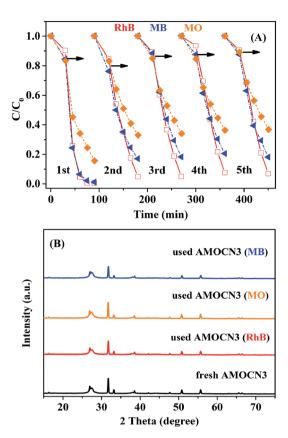
Fig. 8 (A) Cycling runs in photocatalytic degradation of RhB, MO or MB over AMOCN3 (30 mg) under visible light irradiation; (B) XRD patterns of AMOCN3 before and after respective photocatalytic reactions.
