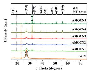
Fig. 1 XRD patterns of T-CN (thin  $g-C_3N_4$  nanosheets), AMOCN1, AMOCN2, AMOCN3, AMOCN4, AMOCN5, and AMO (β-Ag<sub>2</sub>MoO<sub>4</sub>).
