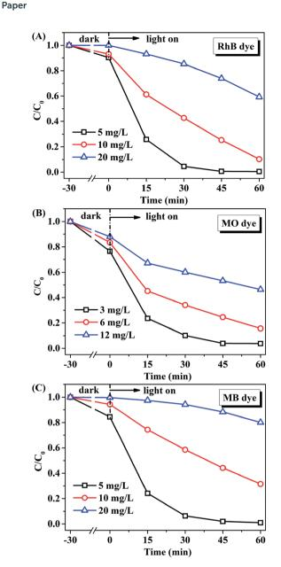
Fig. 7 The effect of initial concentration of (A) RhB, (B) MO or (C) MB on the catalytic performance of AMOCN3 (30.0 mg) under visible light irradiation.
