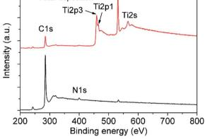
Fig. 3 Raman (a) and XPS spectra (b) of the structures before and after electrophoretic deposition of  $TiO_2$  nanoparticles.
