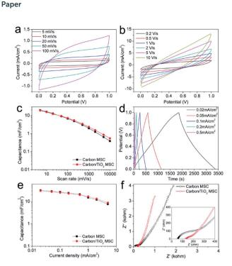
Fig. 4 Electrochemical properties of the carbon/TiO<sub>2</sub> composite electrode. CV curves at low scan rate (a) and high scan rate (b), specific capacitance calculated from CV data as a function of scan rate (c), CC curves (d), specific capacitance calculated from CC data as a function of current density (e), and Nyquist plots of MSCs before and after TiO<sub>2</sub> deposition (f). The inset in (f) shows the high-frequency region of the Nyquist plots.
