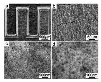
Fig. 2 Large-scale (a and b) and enlarged SEM images (c and d) of the carbon/ $TiO_2$  composite electrode obtained by laser direct writing on PI film in Ar and following electrophoretic deposition of  $TiO_2$  nanoparticles.
