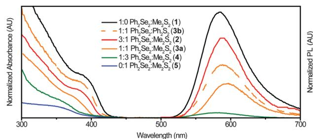
**Fig. 2** Absorption (left) and PL (right) spectra of  $\text{Mn}^{2+}:\text{ZnSe}_{1-x}\text{S}_x$  NCs with varying dichalcogenide precursor ratios. The NC first absorption peak shifts from  $\sim 390$  nm for  $\text{Ph}_2\text{Se}_2$  alone (1) to a broad feature at  $\sim 340$  nm for  $\text{Me}_2\text{S}_2$  alone (5). The PL peak red-shifts from 586 nm to 589 nm with increasing S. For 4, very little luminescence was detected and for 5 no luminescence was detected.
