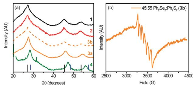
Fig. 4 (a) XRD patterns of samples **1**, **2**, **3a**, **3b**, and **4**. The patterns indicate zinc-blende structure and the broadness of the peaks indicates small NC diameters or domains. As the amount of S increases, the peaks shift to larger angles. The black lines at the bottom of the figure represent the positions of bulk ZnSe and the blue lines represent those of bulk ZnS. (b) EPR spectrum of **3b** showing a splitting pattern with 6 peaks and a hyperfine coupling constant of 66.2 G.
