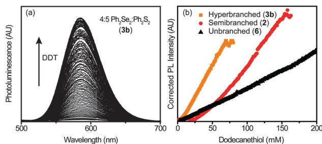
Fig. 5 (a) Steady-state PL of **3b** in the presence of dodecanethiol (DDT). Increasing the amount of thiol leads to a concomitant increase in  $\text{Mn}^{2+}$  PL from the NCs. (b) Scatter plot of the  $\text{Mn}^{2+}$  PL intensity *vs.* [DDT] for NC samples with different degrees of branching. The more branched **3b** NCs show the steepest increase in PL intensity with thiol. NCs with less (**2**) and no (**6**) branching show decreasing sensitivity to thiol, with smaller increases in slope.
