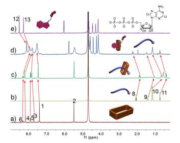
Fig. 7  $\,^{1}$ H NMR spectra (500 MHz, D<sub>2</sub>O, 298 K): (a) 3.00 mM 1; (b) 3.00 mM 2; (c) 1 and 2 (3.00 mM for each); (c) 1, 2, and ATP (3.00 mM for each); (e) 3.00 mM ATP.
