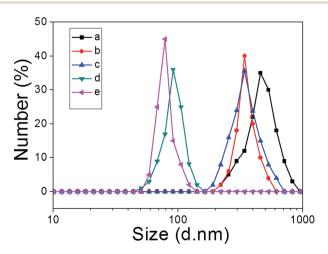
Fig. 4 DLS data corresponding to the copolymer aggregates (0.500 mM) produced upon the addition of different amounts of 1 (mM): (a) 0; (b) 0.500; (c) 1.00; (d) 1.50; (e) 2.30 to copolymer 3.
