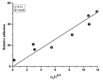
Fig. 4 The relationship between relative adhesion and the square root of the product of critical surface energy  $\gamma_{\rm c}$  and  $\it E$  modulus for polymers to be used in AF surfaces. Redrawn from data in ref. 46. The inset numbers correspond to the polymers listed in Table 1
