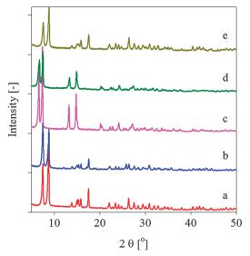
Fig. 1 PXRD patterns of (a) MIL-140A-MW, (b) MIL-140A-CE, (c) MIL-140B-MW, (d) MIL-140B-CE and (e) MIL-140A-NH<sub>2</sub>-MW.
