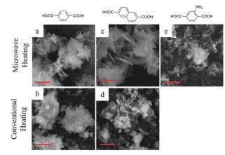
Fig. 2 SEM images of (a) MIL-140A-MW, (b) MIL-140A-CE, (c) MIL-140B-MW, (d) MIL-140B-CE and (e) MIL-140A-NH<sub>2</sub>-MW (scale bar =  $3 \mu m$ ).
