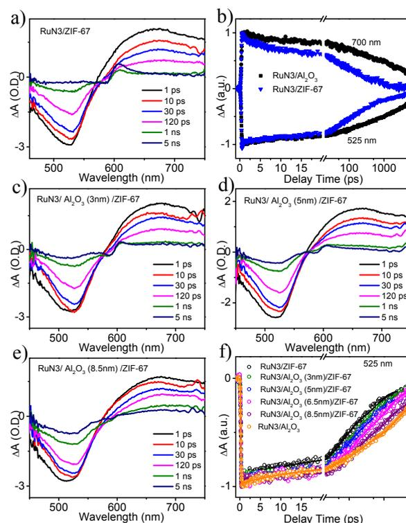
**Figure 2.** Transient absorption spectra of RuN3/ZIF-67 (a), RuN3/ $\text{Al}_2\text{O}_3(3\text{nm})$ /ZIF-67 (c), RuN3/ $\text{Al}_2\text{O}_3(5\text{nm})$ /ZIF-67 (d), and RuN3/ $\text{Al}_2\text{O}_3(8.5\text{nm})$ /ZIF-67 (e); b) the comparison of GSB recovery and ESA decay kinetics of RuN3 on ZIF-67 and  $\text{Al}_2\text{O}_3$ ; f) The comparison of GSB recovery kinetics of RuN3 on different substrate.
