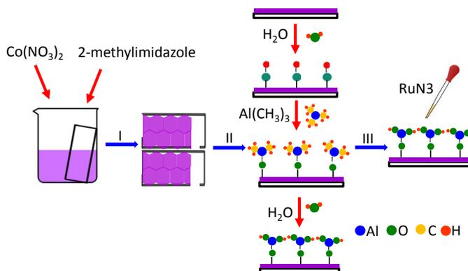
**Scheme 1.** Schematic representation of the synthesis of RuN3/Al<sub>2</sub>O<sub>3</sub>/ZIF-67 thin film.
