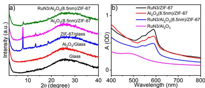
**Figure 1.** a) XRD patterns of glass,  $\text{Al}_2\text{O}_3$ /glass, ZIF-67/glass,  $\text{Al}_2\text{O}_3(8.5\text{nm})$ /ZIF-67 and RuN3/ $\text{Al}_2\text{O}_3(8.5\text{nm})$ /ZIF-67; b) UV-visible absorption spectra of RuN3/ZIF-67,  $\text{Al}_2\text{O}_3(8.5\text{nm})$ /ZIF-67, RuN3/ $\text{Al}_2\text{O}_3(8.5\text{nm})$ /ZIF-67 and RuN3/ $\text{Al}_2\text{O}_3(8.5\text{nm})$ .
