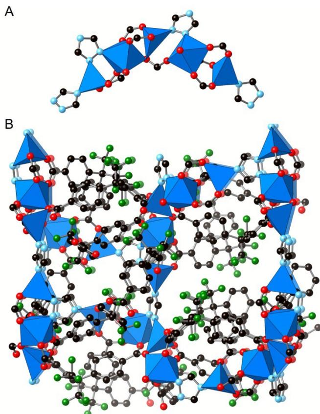
**Figure 3.** A) The inorganic SBUs in TMPF-95 are composed of five V-shaped disposed polyhedral metal cations. B) Representation of three dimension structure of TMPF-95. Carbon is black, oxygen is red, fluorine is green and nitrogen is cyan. Blue polyhedra represent metal (Zn, Co) cations. Hydrogen atoms are omitted for clarity.
