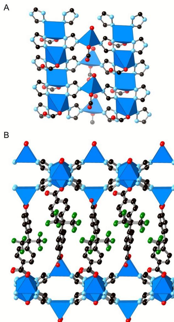
**Figure 2.** A) The inorganic SBU in TMPF-91 can be depicted as rods of metal cations, which are linked by triazolate anions. B) Representation of the three dimensional structure of the TMPF-91 along *c* axis. Layers depicted in A are perpendicular to the figure, and are connected by hfipbb<sub>2</sub> linkers. Carbon is black, oxygen is red, fluorine is green and nitrogen is cyan. Blue polyhedra represent metal (Zn, Co) cations. Hydrogen atoms are omitted for clarity.
