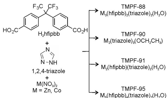
**Scheme 1:** Combination of the 4,4'-hexafluoroisopropylidenebisbenzoic acid (H<sub>2</sub>hfipbb), 1,2,4-triazole and zinc and cobalt nitrate salts results in the formation of four new MOFs. In the MOF formulae, M might stand for Zn, or a mixture of Zn and Co at various ratios, as explained in the text.
