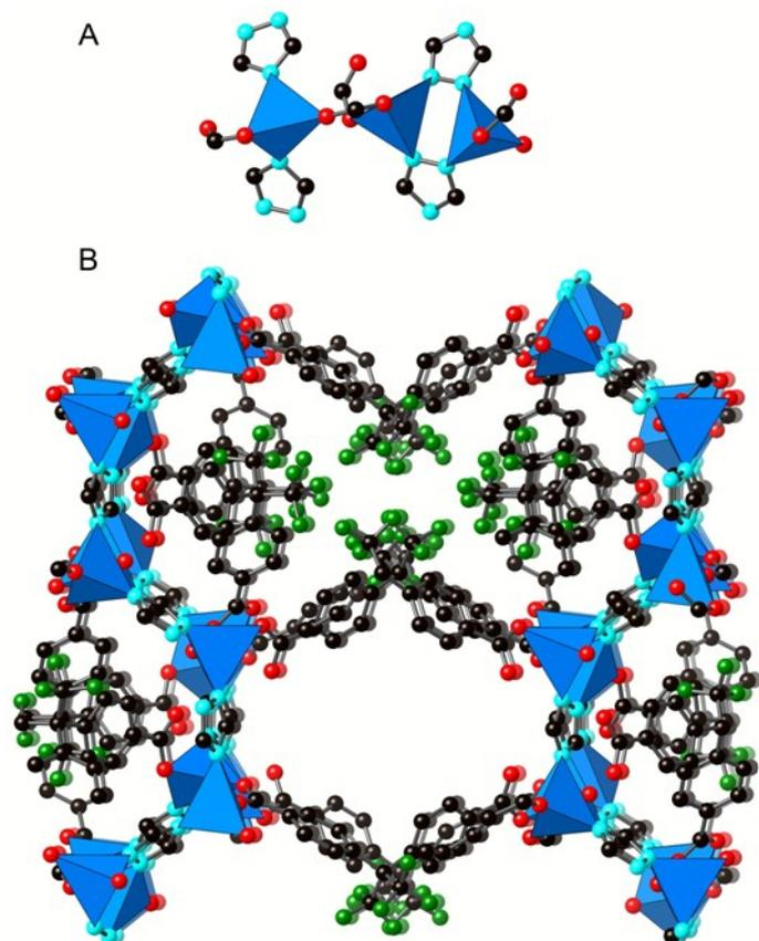
**Figure 1.** A) The inorganic SBU in TMPF-88 is composed of three linearly disposed tetrahedral metal cations. B) Depiction of TMPF-88, viewed along the *c* axis. Carbon is black, oxygen is red, fluorine is green and nitrogen is cyan. Blue polyhedra represent metal (Zn, Co) cations. Hydrogen atoms are omitted for clarity.
