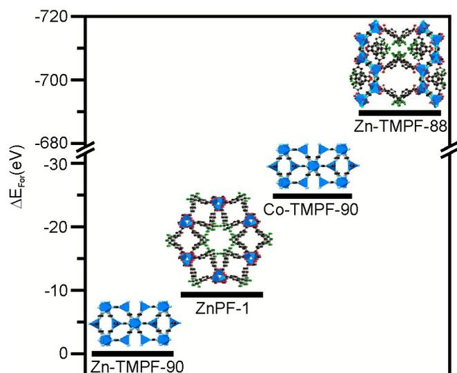
**Figure 9.** Relative formation energies for the phases involved in the kinetic study.  $\Delta E_{\text{Form}}$  values have been normalized to the most stable phase.
