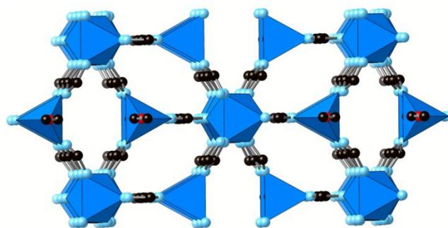
**Figure 4.** Structural representation of TMPF-90 viewed along  $a$  axis. Carbon is black, oxygen is red and nitrogen is cyan. Blue polyhedra represent metal (Zn, Co) cations. Hydrogen atoms are omitted for clarity.
