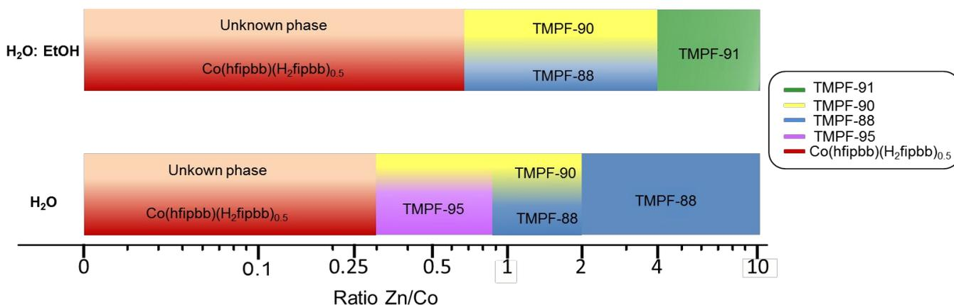
**Figure 5.** The phase diagram for the obtained products with varying Zn/Co ratios, in two different conditions: water:ethanol (up) and water (down). For all experiments, temperature was 170 °C, and heating time 18h. The Zn/Co ratio is shown in logarithmic scale, indicating the values that were investigated.
