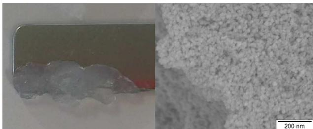
Amorphous calcium oxalate nanoparticles with sizes of 10-30 nm were synthesized at room temperature by the hydrolysis of a dimethyl oxalate from ethanol solution.
