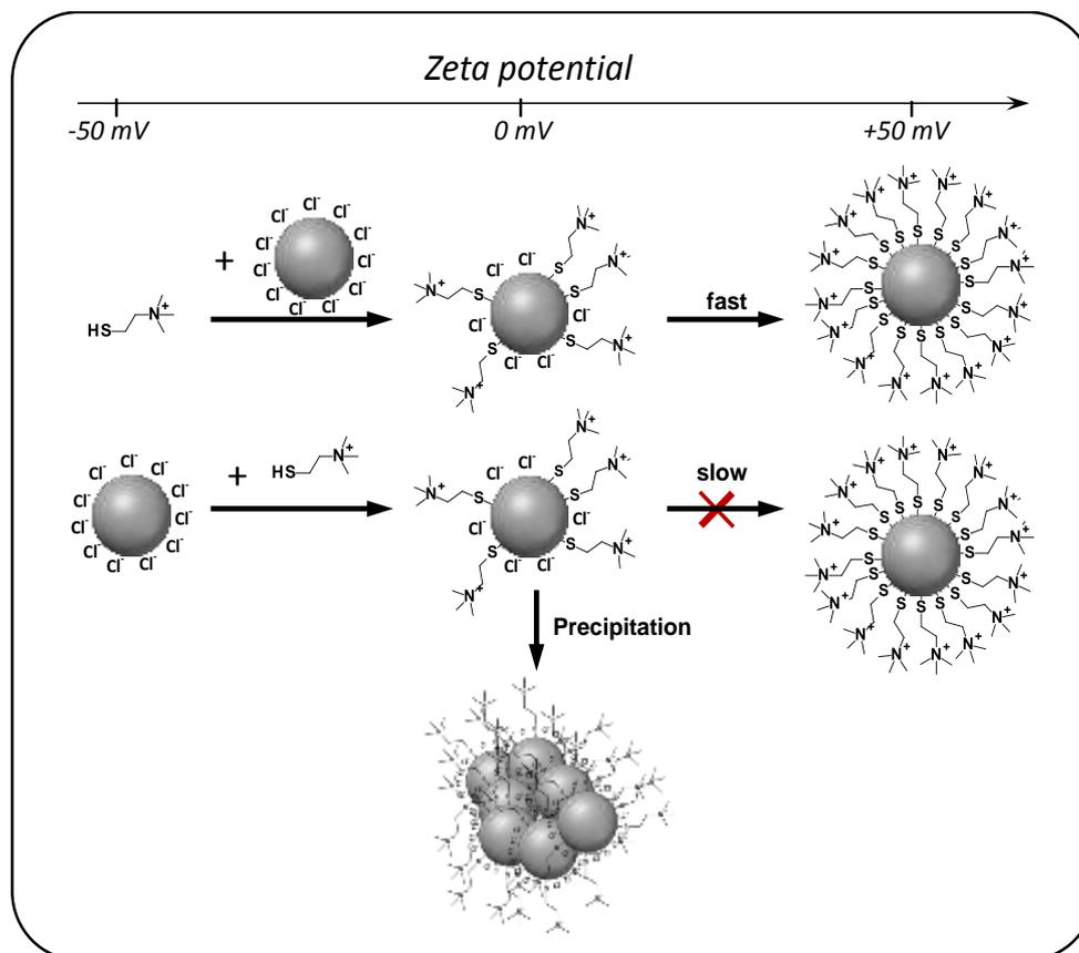
**Scheme 1.** Schematic showing how adding thiocholine (TC) to a silver colloid results in a low effective concentration and charge neutrality on the surface (a). Slowly adding colloid to thiocholine gives a high effective concentration of modifier and overcomes charge neutrality (b).
