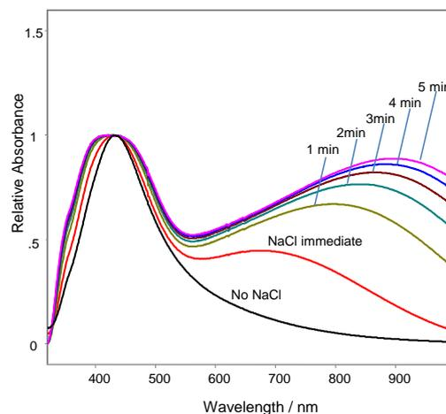
**Figure 3.** UV/vis spectra of HRSC+ over a period of 5 minutes when NaCl is added.
