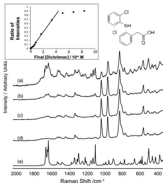
**Figure 5.** SERS spectra of different concentrations of diclofenac adsorbed onto HRSC+ and aggregated with 0.1 M MgSO<sub>4</sub>. Concentration of diclofenac is (a)  $8.3 \times 10^{-4}$  M, (b)  $8.3 \times 10^{-5}$  M, (c)  $5 \times 10^{-5}$  M, (d) 0. Spectrum (e) is a normal Raman spectrum of diclofenac sodium powder for reference. Spectra have been scaled and vertically offset for clarity. Inset shows a plot of the intensity ratio of diclofenac/TC marker bands against [diclofenac].
