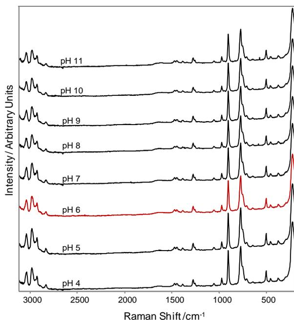
**Figure 2.** Raw SERS spectra of HRSC+ at varying pH values. The pH was adjusted using HCl or NaOH, before drawing 200  $\mu$ L aliquots and aggregating with 20  $\mu$ L 1 M NaCl. Spectra have been vertically offset for clarity, but are displayed on the same scale and are completely unprocessed. The pH 6 spectrum is highlighted as the typical pH of HRSC+ without adjustment.
