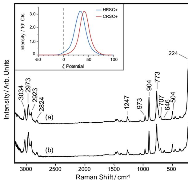
Figure 1. SERS spectra of (a) HRSC+ and (b) CRSC+. Inset shows the  $\zeta$  potential distribution for each colloid.
