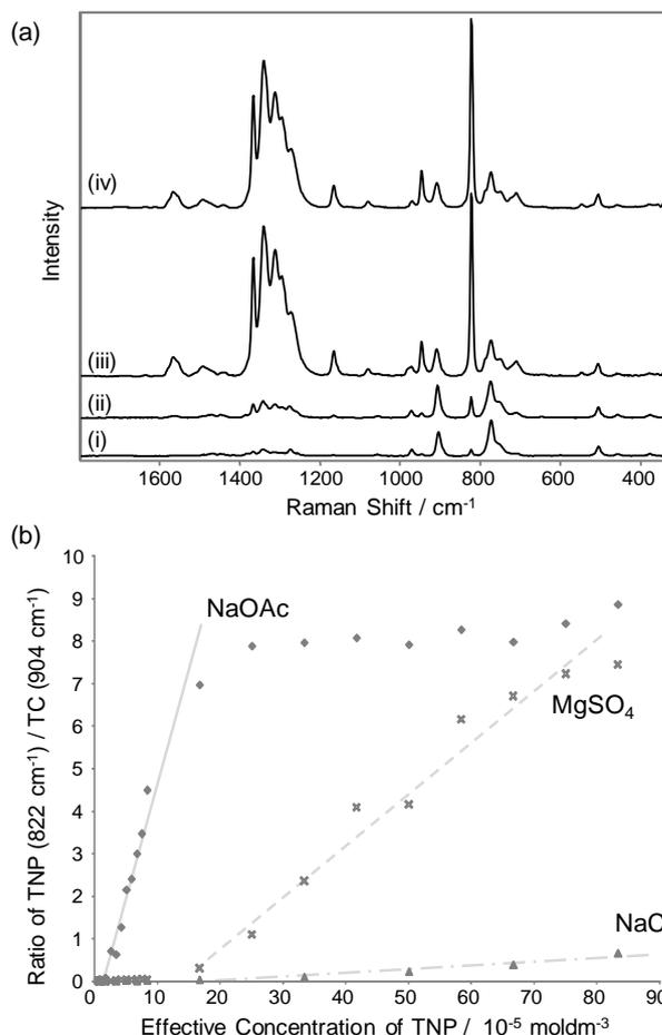
**Figure 4.** (a) Spectra obtained when  $3.6 \times 10^{-4}$  M picric acid was added to HRSC+ and aggregated with (i) 1 M KBr, (ii) 1 M NaCl, (iii) 0.01 M  $\text{MgSO}_4$ , and (iv) 1 M NaOAc. Spectra have been normalized to the  $774 \text{ cm}^{-1}$  band of thiocholine. (b) Change in picric acid signal with concentration when using different aggregating agents, 1 M NaCl, 0.01 M  $\text{MgSO}_4$  and 1 M NaOAc.
