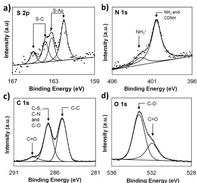
Figure 3. XPS spectra of the a) S 2p, b) N 1s, c) C 1s and d) O 1s peak regions of **biotin-4KC:C11TEG** mixed SAMs at a 1:40 solution ratio.
