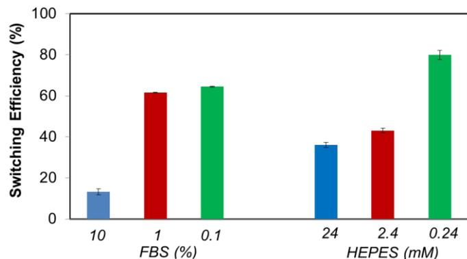
Figure 6. Switching efficiency, as determined by SPR analysis under OC conditions and an applied negative potential ( $-0.4$  V), on **biotin-4KC:C11TEG** mixed SAMs which were exposed to neutravidin in FBS and HEPES. The switching efficiency of the different media was tested at different dilutions in PBS buffer. Error bars show standard deviations among three different substrates.
