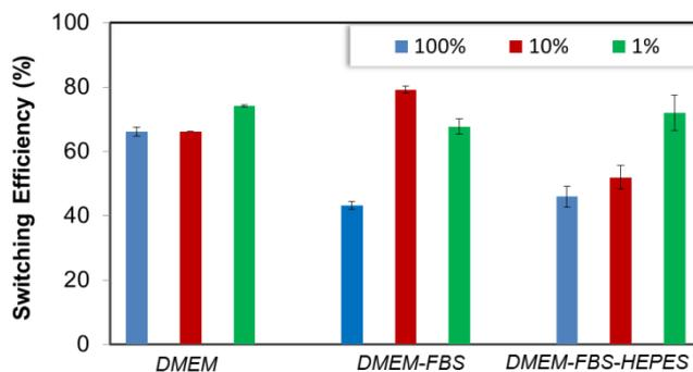
Figure 5. Switching efficiency, as determined by SPR analysis under OC conditions and an applied negative potential ( $-0.4$  V), on **biotin-4KC:C11TEG** mixed SAMs which were exposed to neutravidin in a) DMEM, DMEM-FBS, DMEM-FBS-HEPES. The switching efficiency of the different media was tested at different dilutions in PBS buffer. Error bars show standard deviations among three different substrates.
