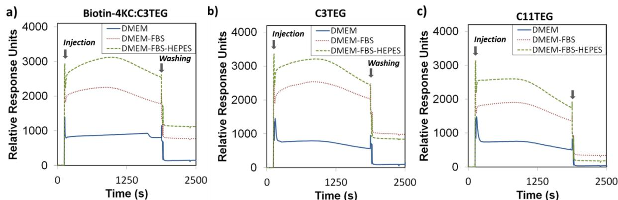
Figure 2. SPR sensorgram traces for the interaction of a) biotin-4KC:C3TEG, b) C3TEG and c) C11TEG SAMs with different complex media – DMEM, DMEM-FBS, and DMEM-FBS-HEPES. The two arrows in the graphs indicate the point of injection of media and PBS washing buffer, respectively.
