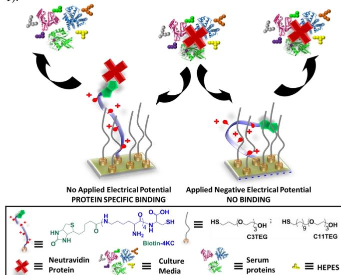
Figure 1. Schematic of the dynamic oligopeptide SAM proposed for controlling specific biomolecular interactions under complex biological conditions. Below: Chemical structures of the oligopeptide (Biotin-4KC) and oligo(ethylene glycol) thiols (C3TEG and C11TEG) used for SAM preparation.
