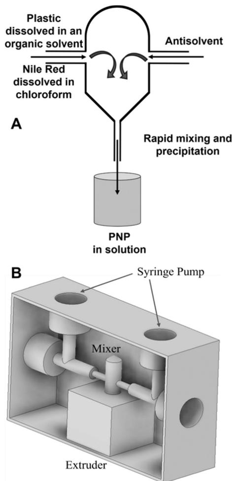
**Fig. 1** Flash nanoprecipitation for preparing fluorescent PNPs. (A) Schematic of the rapid mixing process, where a mixture of plastics (dissolved in an organic solvent) and NR dye (dissolved in chloroform) is introduced in the CIJ-D mixer along with an antisolvent, leading to the instantaneous precipitation of fluorescent PNPs. (B) CAD rendering of custom-built CIJ-D mixer.
