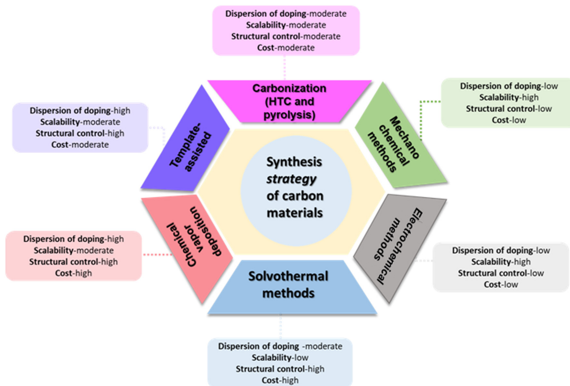
Fig. 4 Comparison of synthetic routes to heteroatom-doped carbons summarising doping efficiency, scalability, and cost.
