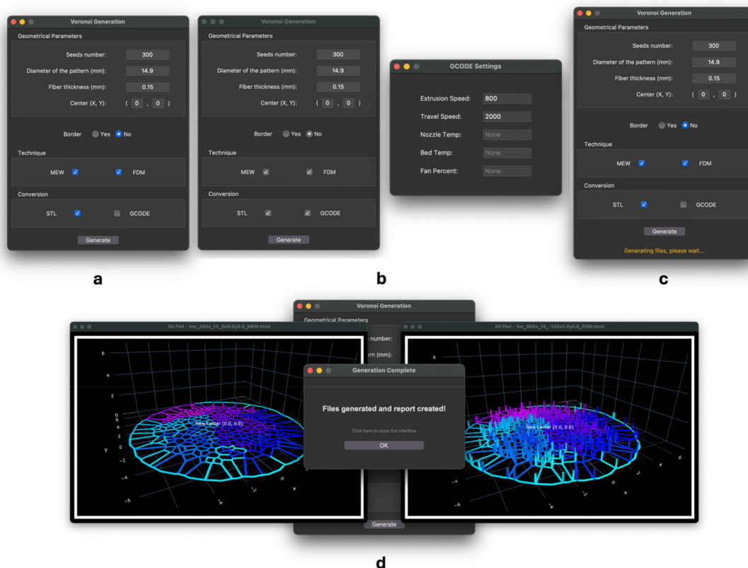
Fig. 3 GUI visualization: (a) starting window of the GUI, (b) additional window in case the “GCODE” option is selected, (c) waiting message at the bottom of the window after pressing the “Generate” button, (d) final windows of the GUI, including the three-dimensional visualization of the pathways and the final message of process completion.
