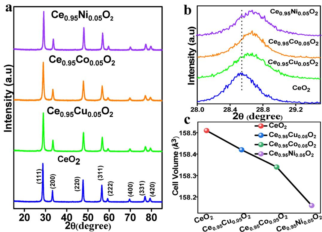
Fig. 2 (a) XRD patterns, (b) zoomed in version, (c) the refined cell volume of  $\text{CeO}_2$  and doped  $\text{Ce}_{0.95}\text{Co}_{0.05}\text{O}_2$ ,  $\text{Ce}_{0.95}\text{Ni}_{0.05}\text{O}_2$ , and  $\text{Ce}_{0.95}\text{Cu}_{0.05}\text{O}_2$ .
